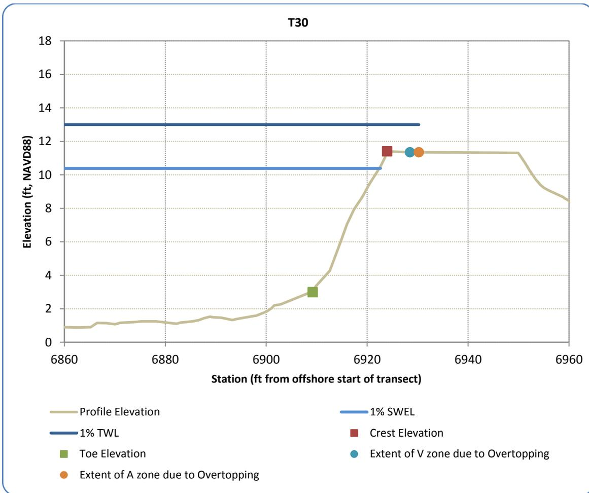
Figure 9. Example of runup and overtopping results showing 1% runup elevation (1% TWL) and overtopping limits for Transect 30
