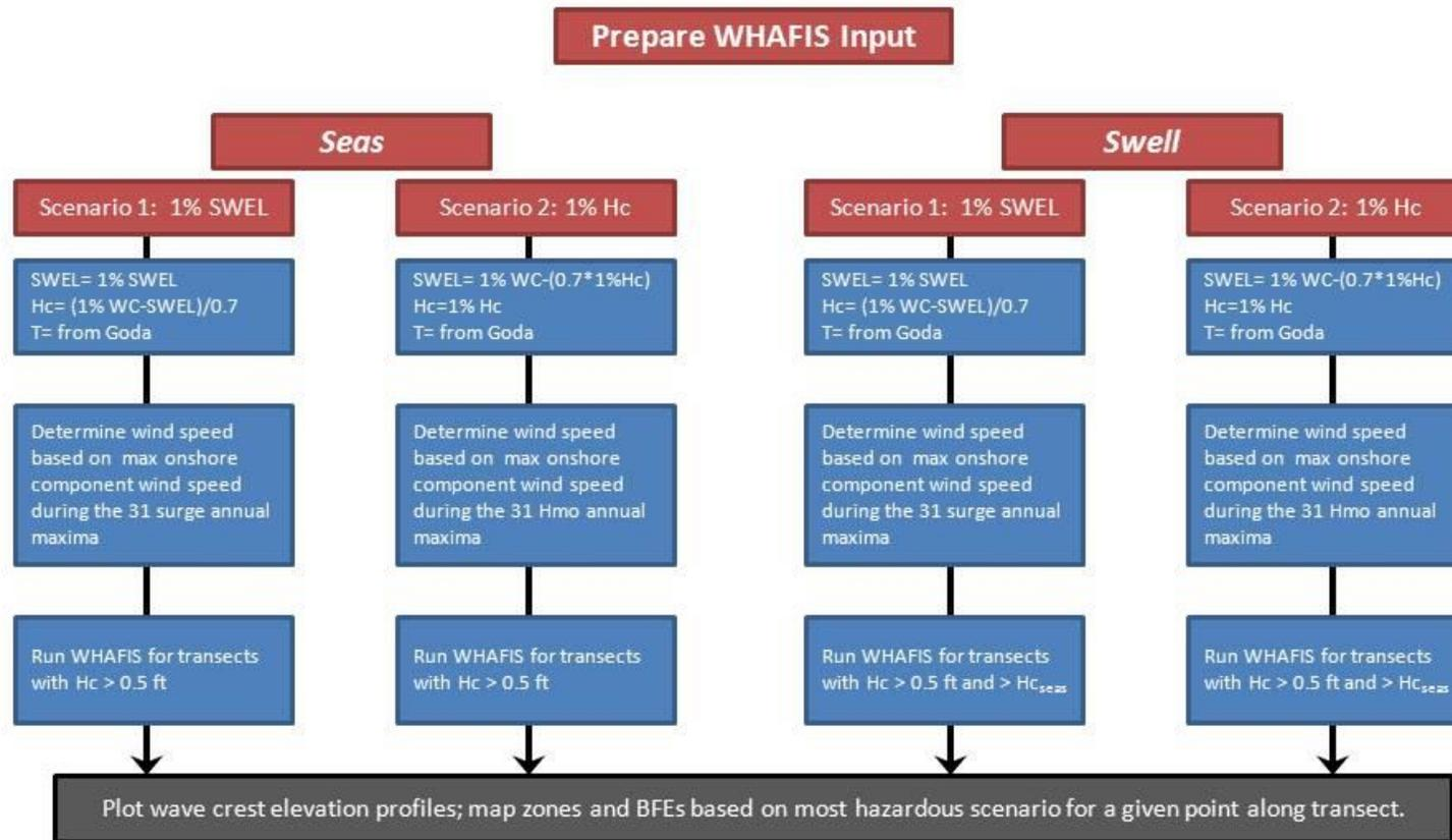
Figure 14. WHAFIS Starting Wave Condition development flow chart
