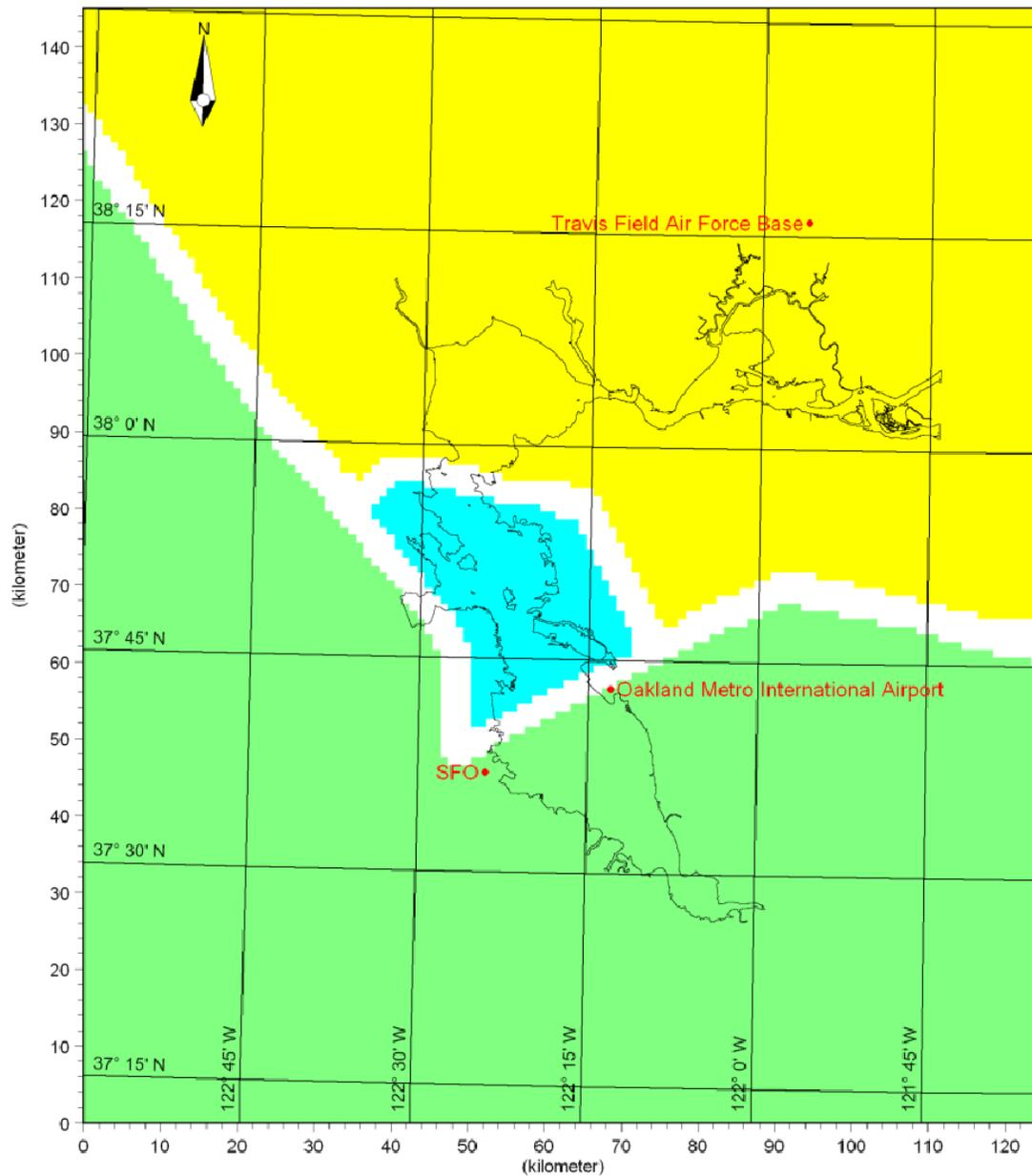
Figure 5. Areas used to assign measured wind data. Yellow area: Travis Field AFB, green area: SFO Airport and cyan area: OAK Airport. White areas indicate transition zones for wind parameters (DHI, 2011)
