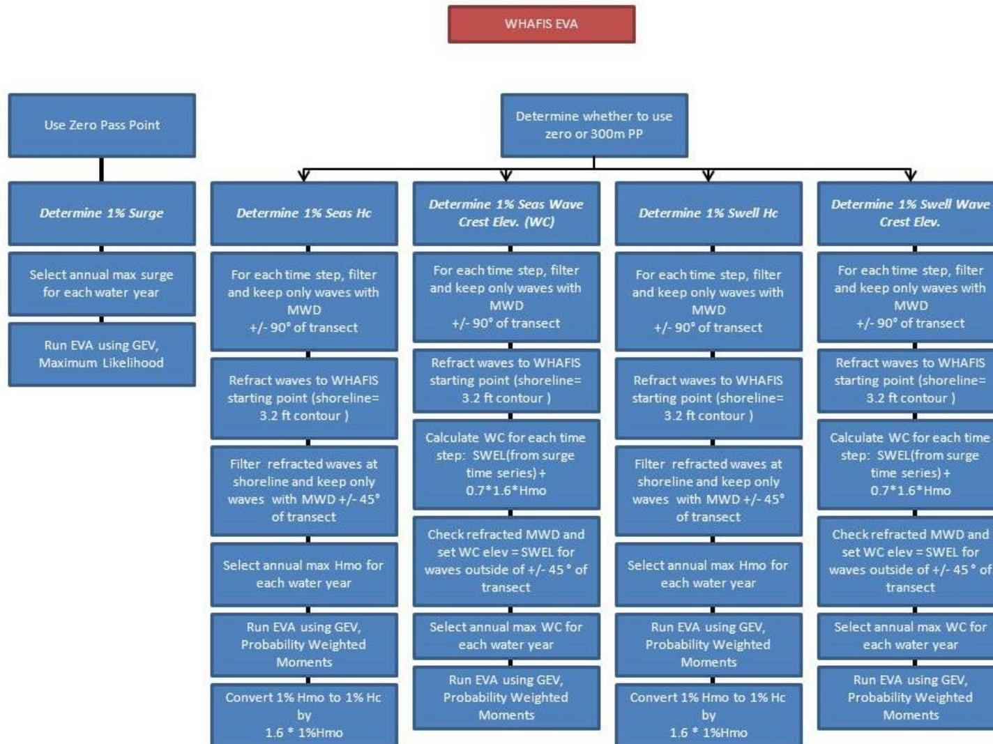
Figure 13. WHAFIS Starting water level and wave condition extreme value analysis flow chart
