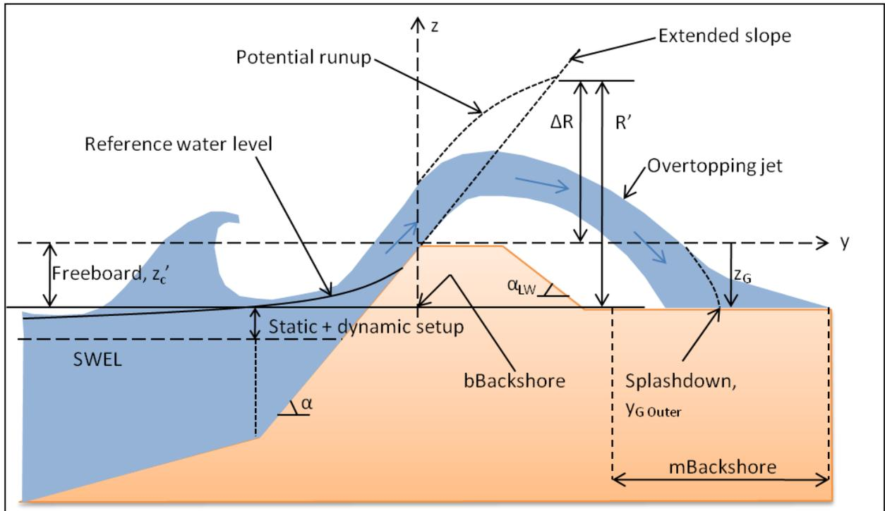
Figure 8. Illustration of splash overtopping and its associated variables
