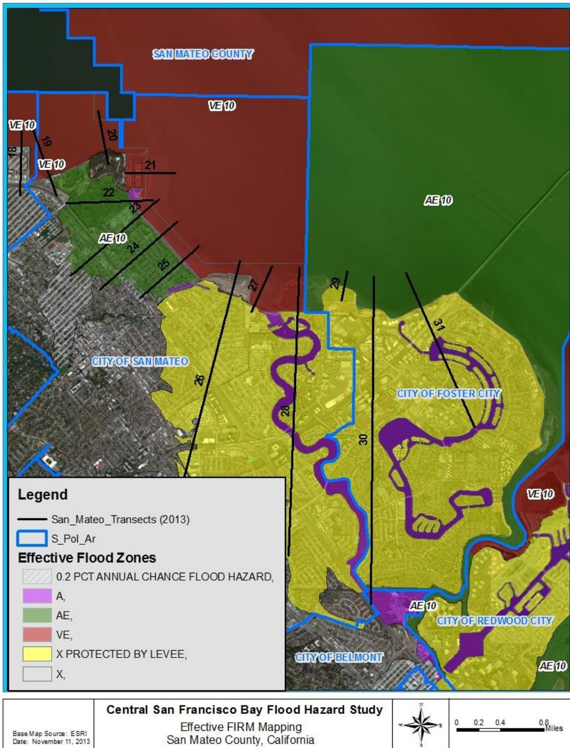
Figure 15. Effective mapping and new study transects in area of interest due to levees
