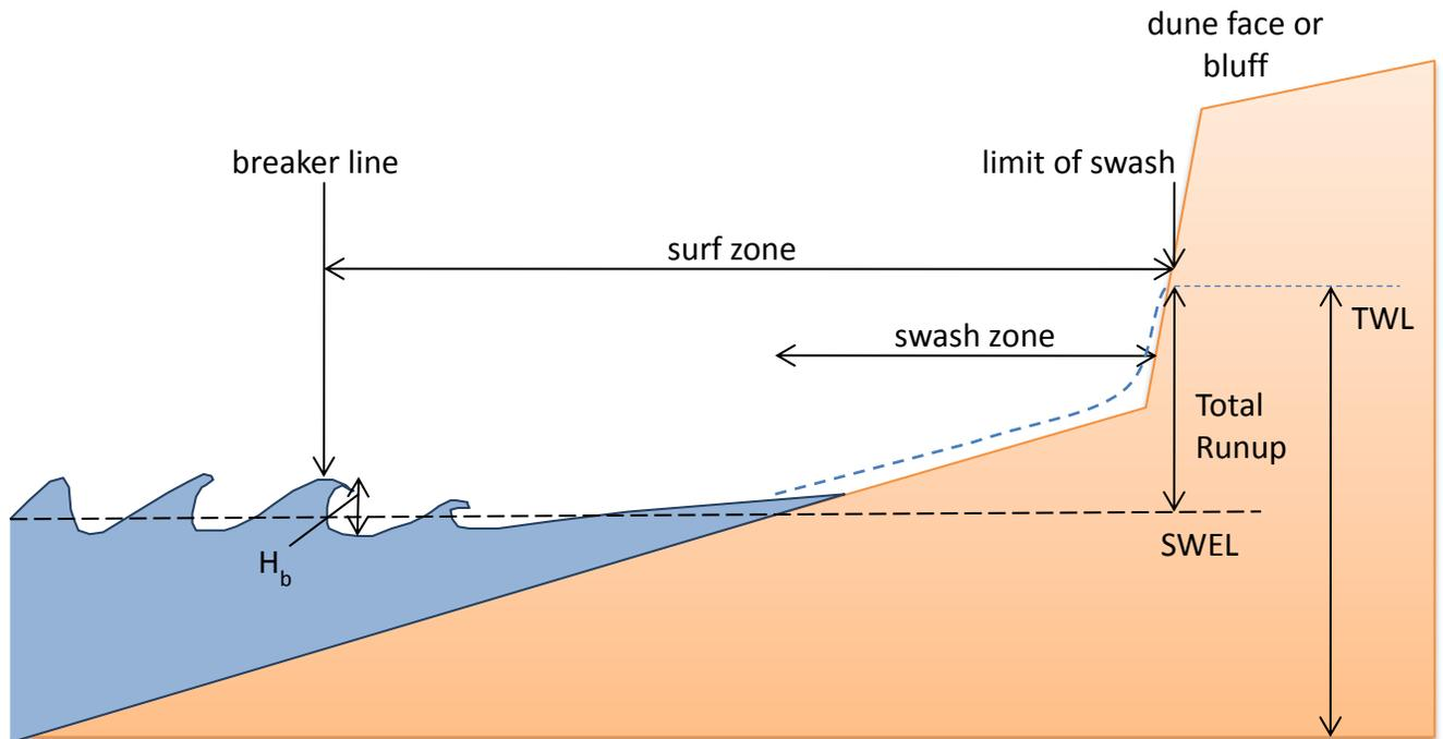
Figure 6. Conceptual model showing the components of wave runup associated with incident waves (modified from Pacific G&S, 2005)
