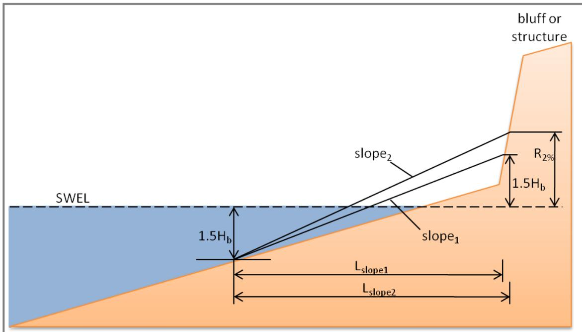
Figure 7. Determination of an average slope based on an iterative approach—first estimate is initially based on  $SWEL \pm 1.5H_{m0}$  (or  $1.5H_b$  where appropriate), and second estimate is the runup limit calculated with the first slope estimate, etc. (modified from van der Meer, 2002)
